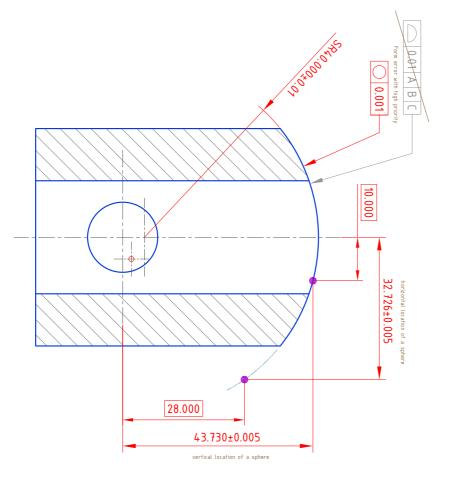
dimension of the tool is within the yields the desired result if the Correction of CNC in several steps tolerance
