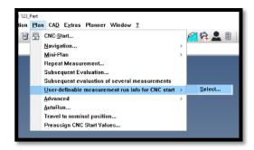
Additionally you can force these operator instructions to appear when they run any pallet or measurement plan. To do this right click a pallet or measuremnt plan select "Define Run Parameters" to modify the run screen. Click the check box "Force Measurement Run Information at CNC Start."
