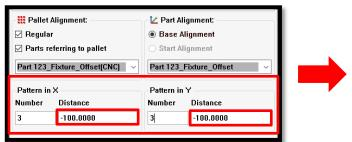
In addition to running in a different direction you can also go out of order any way you want with "define loop" do this by right clicking the pallet icon.
