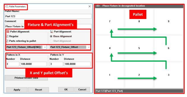
Again the benefit to using this method over example 1 is that if your fixture is misplaced or misoriented. All you need to do is rerun your fixture program (or Manual Alignment of the fixture program) and your program will still run and compensate for the tilted fixture.
