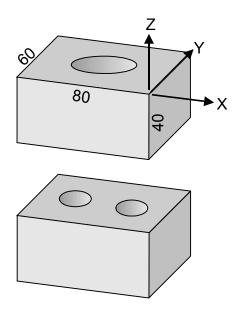
In this way one and the same measurement plan can be used to measure and test different workpieces: for example, a plate with either one or two holes – even if the radii are different. Different geometries, differences in the number of certain features, the presence or absence of features - all these can be parameterized.
