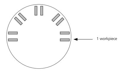
Thus, the number of equal workpieces which can be measured in this way is double the number of parameterized rotary table positions.
