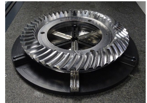
Face plate extension for diameters up to 800 mm
