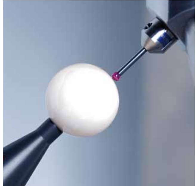
The diameters of the test spheres and the stylus tips are specified in ISO 10360-4 to enable comparisons of runtimes.
