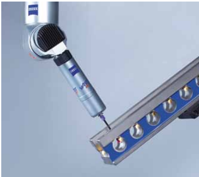
Compared to unidirectional measurements and sphere distance measurements, hysteresis and stylus tip radius errors are included in the results of the two-point distance measurement on the gauge block.
