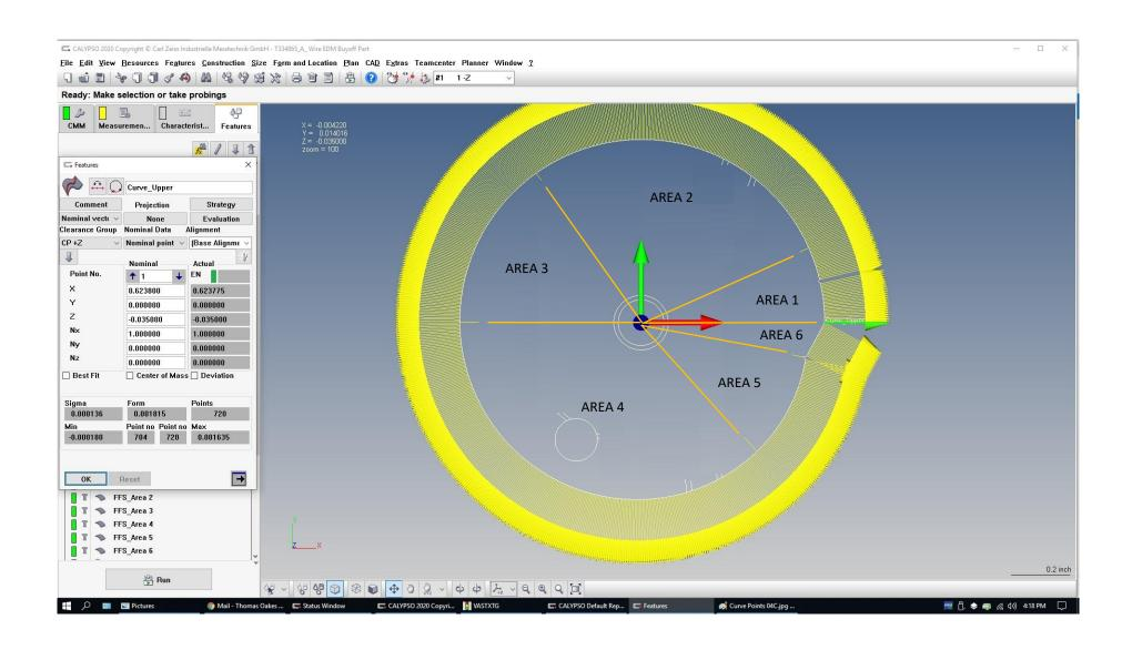
Increased the scanned points to 3 times the number of curve points
