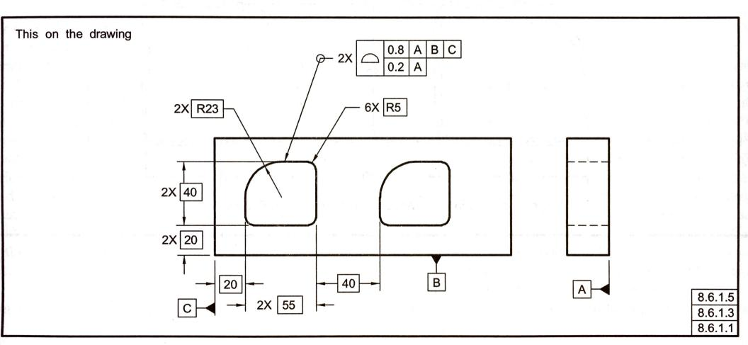
Fig. 8-21 Pattern Located by Composite Profile Tolerancing (Cont'd)
