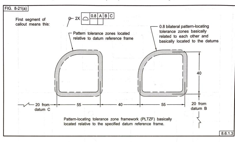
Fig. 8-21 Pattern Located by Composite Profile Tolerancing (Cont'd)
