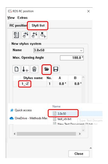
12. Styli list should show all of the stylus names and RDS angles from cmm stylus system. Next, click Create a New Stylus System icon at top.
