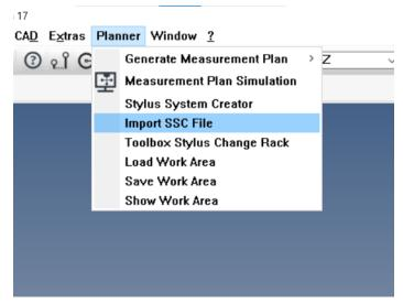
6. On first time only, select Import **SSC MasterProbe**, then select the ssc file designated as MasterProbe. Checkmark signifies success.
