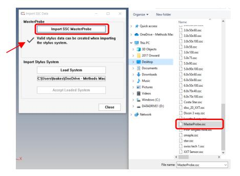
Click Load System, then select the ssc file for desired stylus system that needs updating, then click Accept Loaded System.
