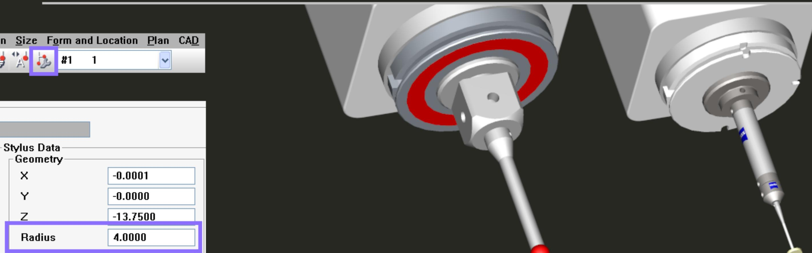
*Using a ring master, compare a measured diameter using the disk probe against the master probe. Adjust the disk radius if needed in the Stylus Management Window*
