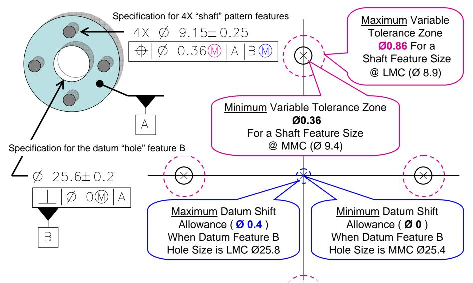
M & D Symbols used in feature tolerance control frames make the feature location or orientation tolerances variable with respect to the feature's size.
