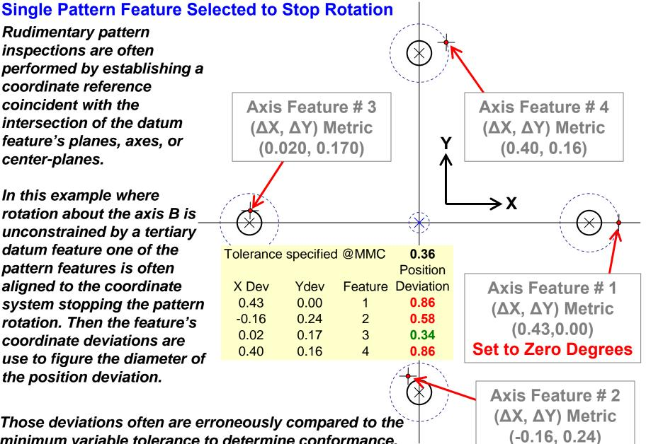
Those deviations often are erroneously compared to the minimum variable tolerance to determine conformance.
