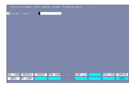
Here the calibration sphere must be probed in the direction of the master probe. The rest of the procedure follows automatically and you cannot influence this.
