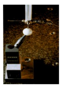
In this case the calibration sphere can be rotated but its position must be redefined.
