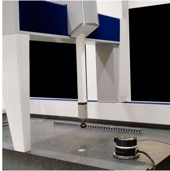
Figure 36 Checking a large CMM with a tracking interferometer (Image © Etalon Ag)
