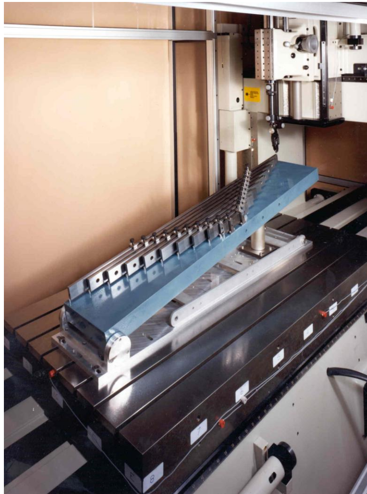
Figure 7 An ISO 10360-2 test being carried out using gauge blocks
