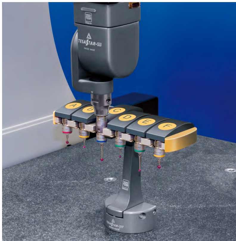
Figure 20 An autochange rack (© Tesa Group)
