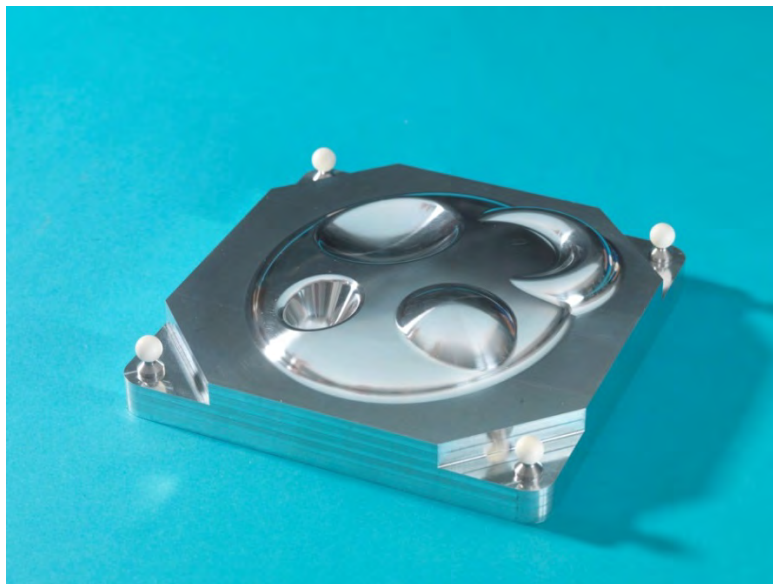
Figure 50 NPL high precision traceable FreeForm reference standard, the standard is available in a number of sizes.
