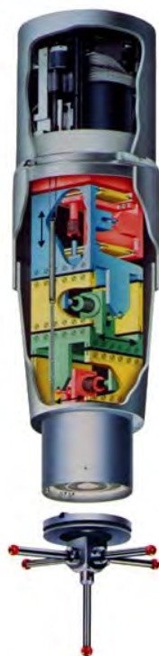
Figure 14 An exploded diagram of an analogue probe head (©Zeiss)
