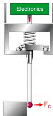
Figure 9 A strain gauge probe mechanism. Note the one of the four silicon strain gauges is shown above the spring in red. Strain gauges trigger at forces that do not unseat the kinematics thus largely eliminating pretravel variation. (© Renishaw plc 2006)
