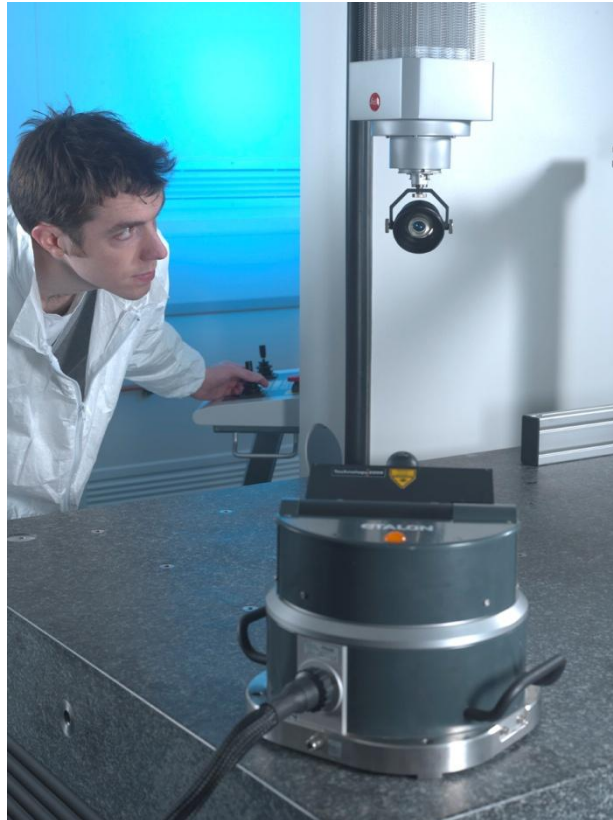
Figure 8 A laser interferometer being used to verify a CMM
