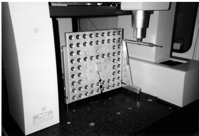
Figure 32 A hole plate being used to check a CMM
