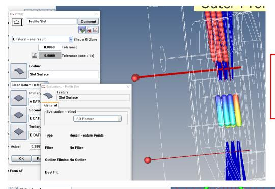
Surface Profile from bad part Recalling Feature Points from 2D Curves into Freeform Surface
