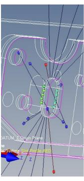
Surface Profile from different bad part Freeform Surface using Faces – if I do this one with Curves, it also gets the Perpendicular points
