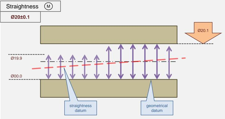
Minimum-feature in order to calculate the straightness. Is not parallel to the geometrical datum.
