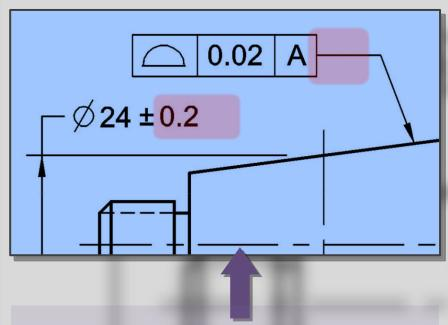
The tolerance-envelope follows the actual surface, only constrained by the cylinder-datum **A**.
