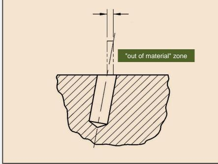
The input of an "out of material" projection zone (P) means a press-fit-situation like shown below.
