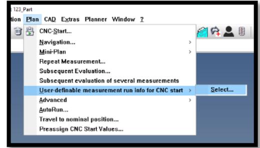
Additionally you can force these operator instructions to appear when they run any pallet or measurement plan. To do this right click a pallet or measurement plan select **“Define Run Parameters”** to modify the run screen. Click the check box **“Force Measurement Run Information at CNC Start.”**
