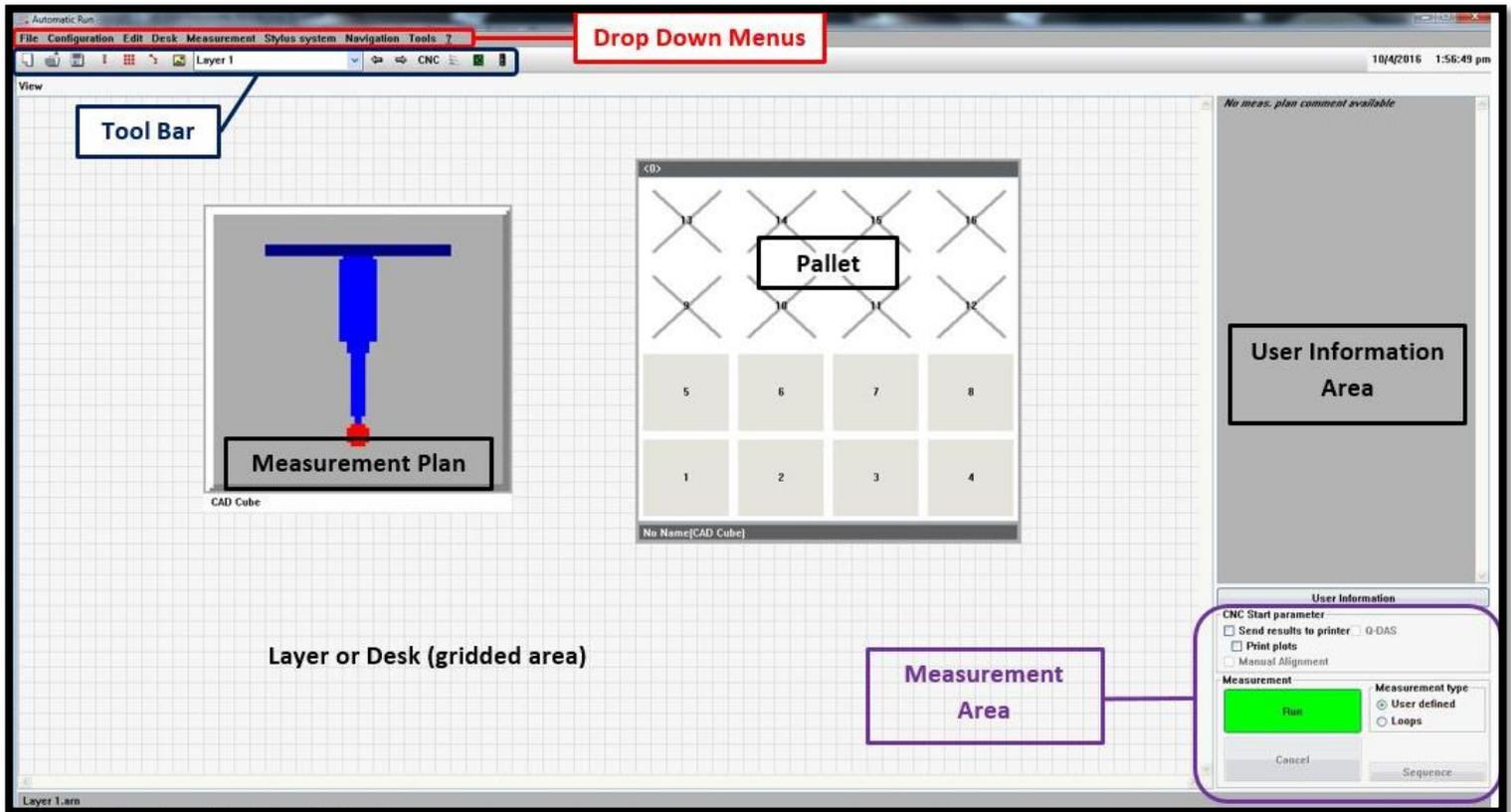
**\*Drop Down Menus:** The Drop-Down Menus allows a variety of AutoRun tasks or even some Calypso tasks (like Stylus System changes) inside the AutoRun Screen.
