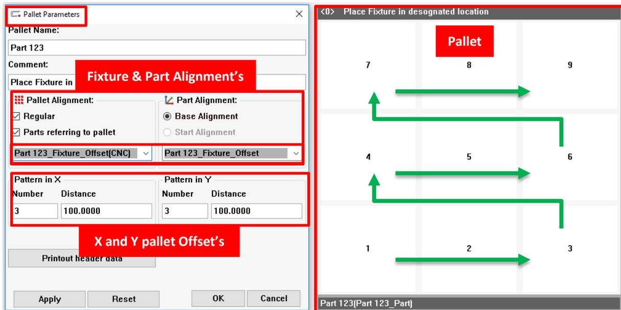
Again the benefit to using this method over example 1 is that if your fixture is misplaced or misoriented. All you need to do is rerun your fixture program (or Manual Alignment of the fixture program) and your program will still run and compensate for the tilted fixture.
