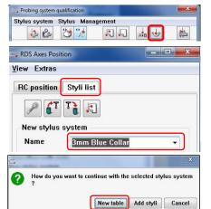
To create the list select Rotate Stylus to New Position and select the Styli List tab, in the RDS Axes Position window. Make sure the newly created Stylus System name is displayed. If the Stylus System Name needs to be changed use the drop down and select the newly created Stylus System. In the new window that opens, select New Table.
