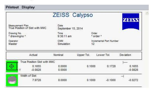
This Report indicates that the Slot is in Tolerance, but shifted to the "right" by 0.0828mm in the rotated coordinate system. Notice that the tolerance WITH BONUS, 0.1728mm, is shown in the "Lower Tol." Column.
