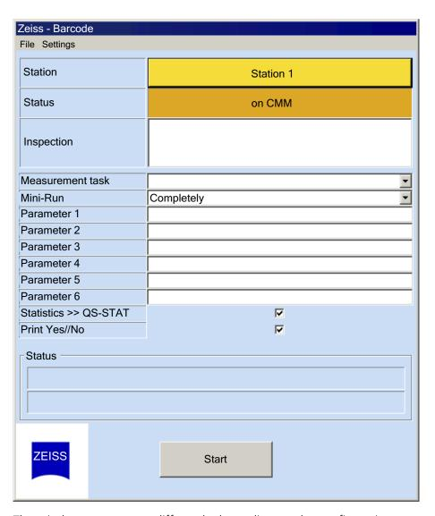
The window may appear differently depending on the configuration: The number of parameters can be set and the check boxes for qs-STAT and printing can be hidden.
