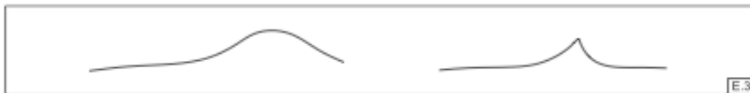
Figure E-3 A Line Which is Tangent Continuous (Left) and Not (Right)
