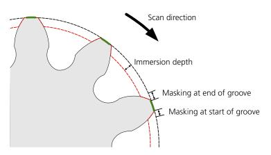
Both the air points at the height of the immersion depth as well as the involute components and points at the start and end of the groove, which would falsify the measuring result due to the approach and retraction movement of the stylus, are masked here.
