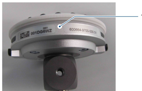
1 Home position of the adapter plate
