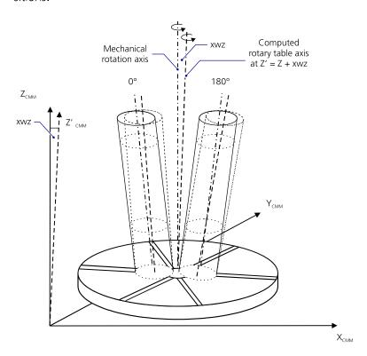
**1** Secure the measurement cylinder onto the rotary table top using, for example, 3-jaw clamps).
